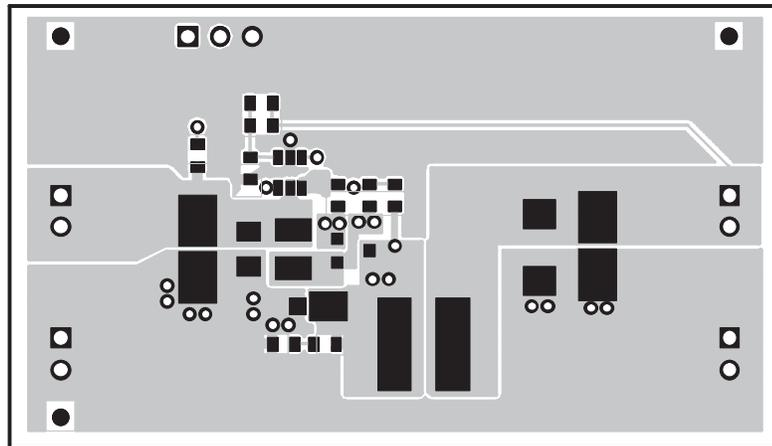
Figure 3-3. Bottom Layer Routing
