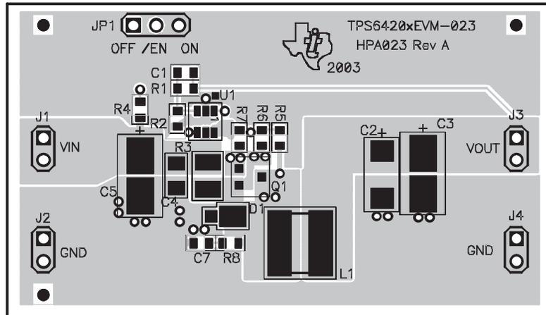
Figure 3–2. Top Layer Routing
