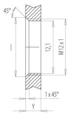
Installation direction: o-ring sits on chamfer.
