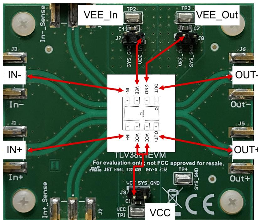
**Figure 3-2. How EVM Designations are Mapped to the TLV3801 Pinout**
