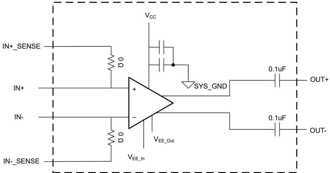
**Figure 7-2. TLV3801 EVM Block Diagram**
