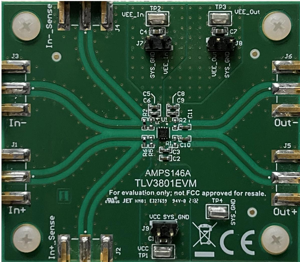
Figure 1-1. TLV3801EVM Board Top View
