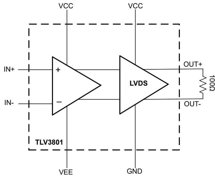
Figure 2-1. TLV3801 Block Diagram
