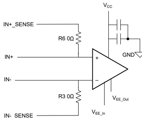
Figure 6-2. Input Side Schematic Without Optional Resistors R4 and R5
