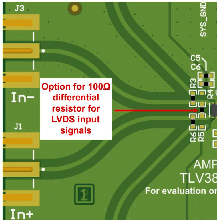
Figure 6-3. Configuration for LVDS Inputs Using the Unused Pads of R4 and R5
