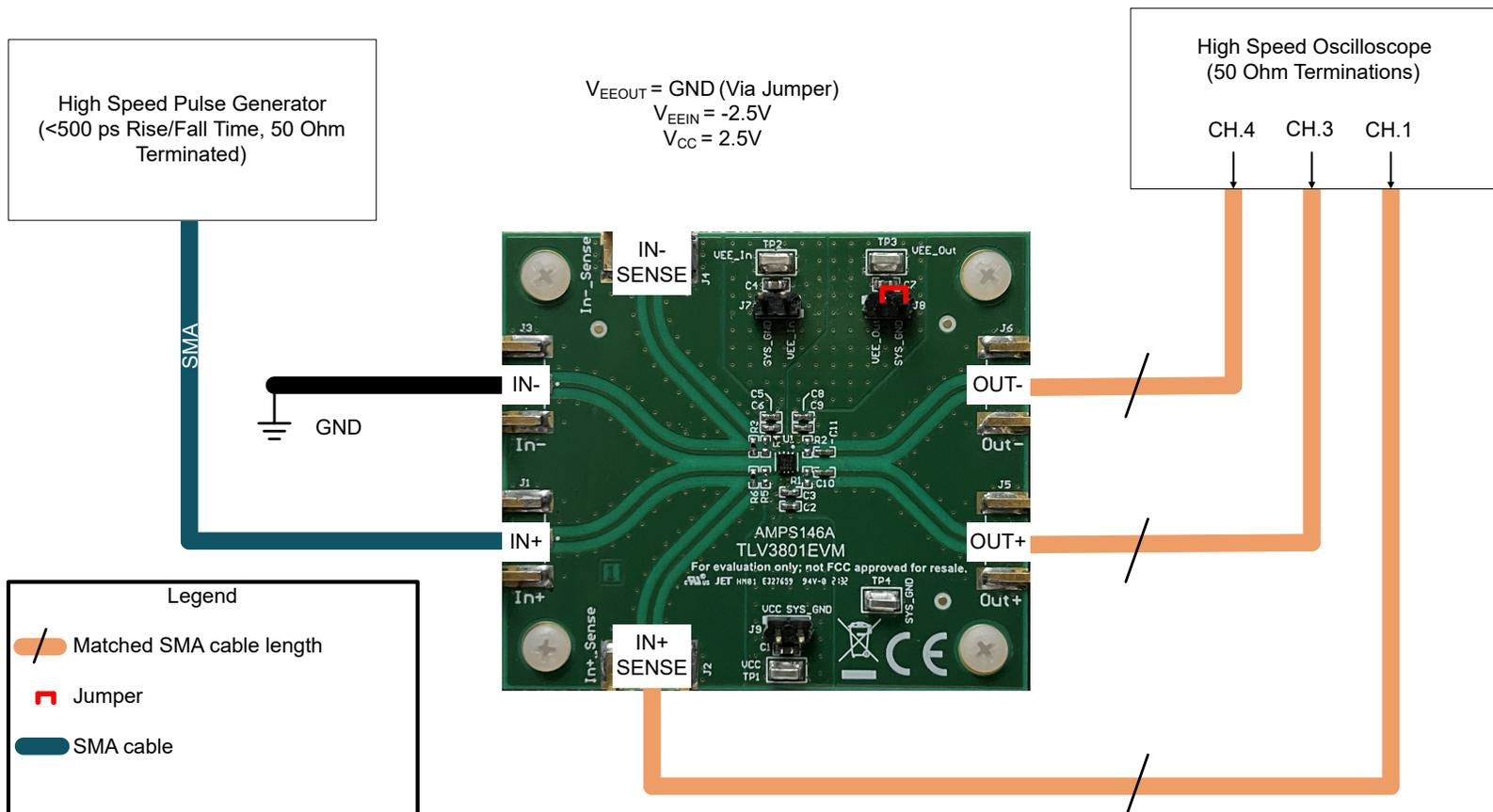
Figure 5-1. TLV3801 EVM Propagation Delay with Latch Setup
