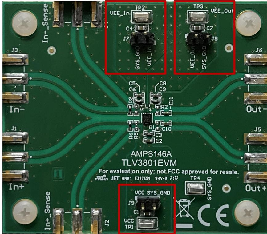
Figure 6-1. TLV3801EVM Supply Voltage Connection
