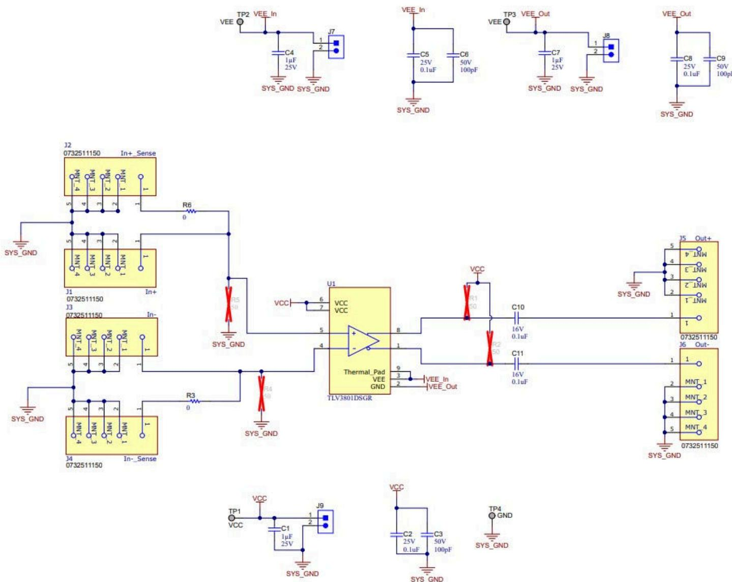
Figure 8-1. TLV3801 EVM Schematic
