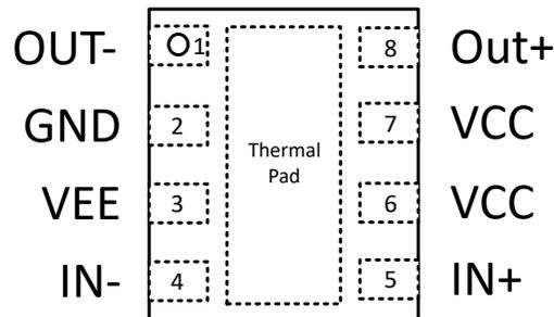
**Figure 3-1. TLV3801EVM Pin Assignments**
