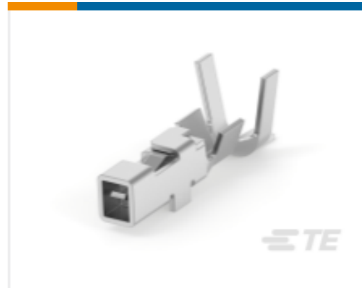
TE Part #1827588-2 Contact: Component To Wire; 3-5A, 30-18 Wire Size
