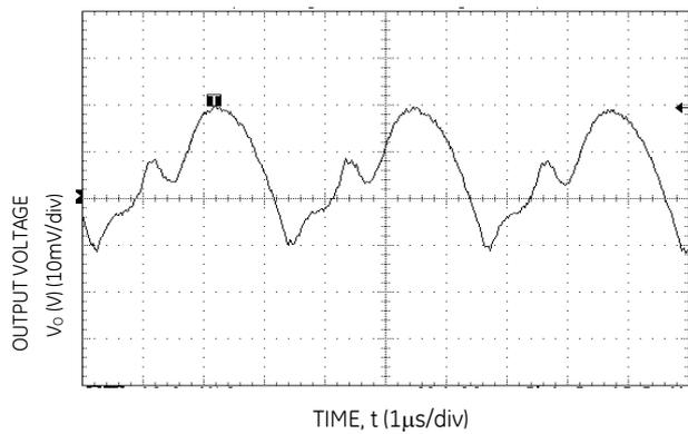
**Figure 9. Typical Output Ripple and Noise**
