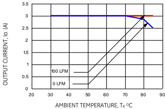
Figure 19. Derating Output Current versus Local Ambient Temperature and Airflow (V<sub>IN</sub> = 12.0 Vdc, V<sub>o</sub>=0.75Vdc).
