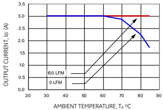
Figure 22. Derating Output Current versus Local Ambient Temperature and Airflow (V<sub>IN</sub> = 12 Vdc, V<sub>o</sub>=5.0 Vdc).
