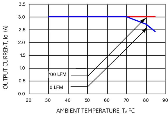
Figure 20. Derating Output Current versus Local Ambient Temperature and Airflow (V<sub>IN</sub> = 12.0Vdc, V<sub>o</sub>=1.8 Vdc).
