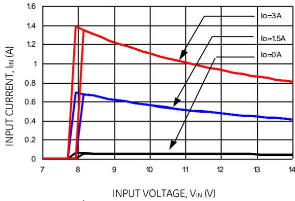
**Figure 7. Input voltage vs. Input Current**
