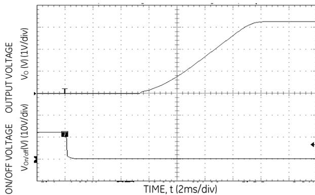
**Figure 15. Typical Start-Up Using Remote On/Off with Low-ESR external capacitors (7x150uF Polymer) ( $V_{in} = 12.0Vdc$ ,  $V_o = 3.3Vdc$ ,  $I_o = 3A$ ,  $C_o = 1050\mu F$ ).**
