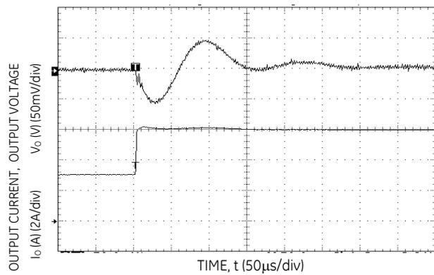
**Figure 12. Transient Response to Dynamic Load Change**
