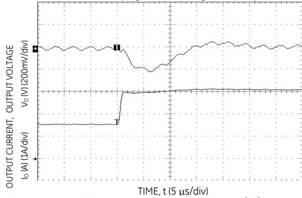
**Figure 10. Transient Response to Dynamic Load Change**
