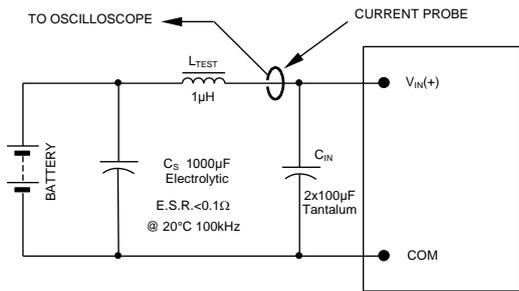
NOTE: Measure input reflected ripple current with a simulated source inductance (L<sub>TEST</sub>) of 1µH. Capacitor C<sub>S</sub> offsets possible battery impedance. Measure current as shown above.
