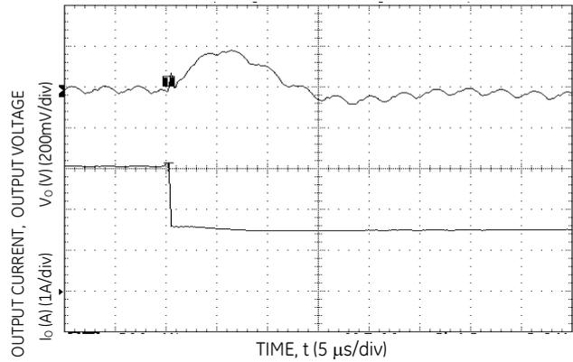
**Figure 11. Transient Response to Dynamic Load Change**
