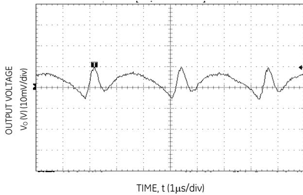
**Figure 8. Typical Output Ripple and Noise**
