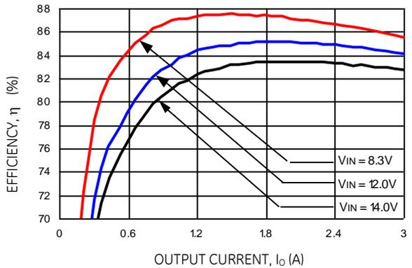
Figure 2. Converter Efficiency versus Output Current (Vout = 1.5Vdc).
