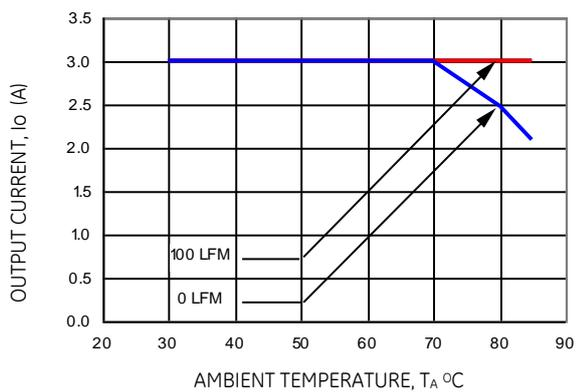
Figure 21. Derating Output Current versus Local Ambient Temperature and Airflow (V<sub>IN</sub> = 12.0Vdc, V<sub>o</sub>=3.3 Vdc).
