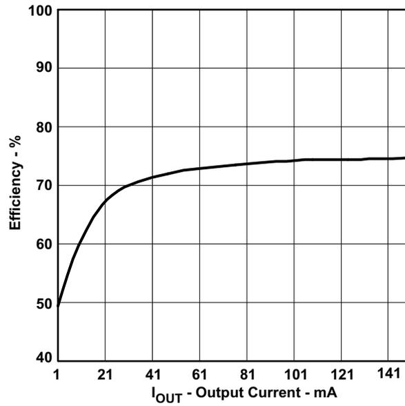
Figure 1. TPS60150 Efficiency with  $V_{IN} = 3.3\text{ V}$
