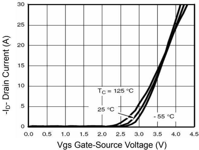
Figure 2 Transfer Characteristics
