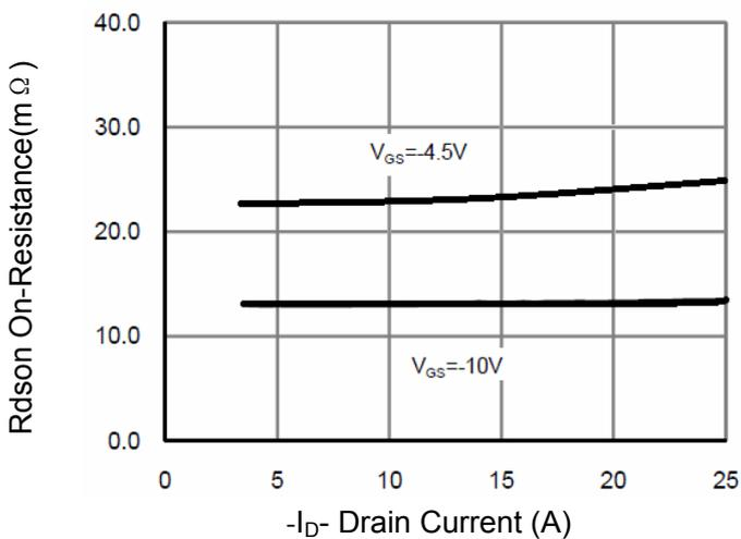
Figure 3 R<sub>dson</sub>- Drain Current
