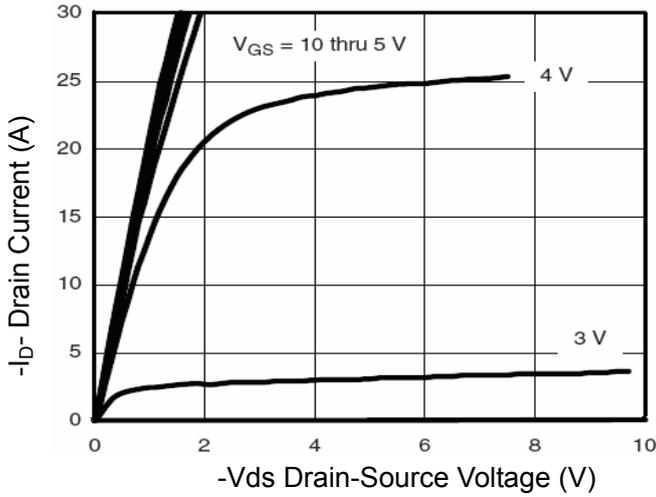
Figure 1 Output Characteristics
