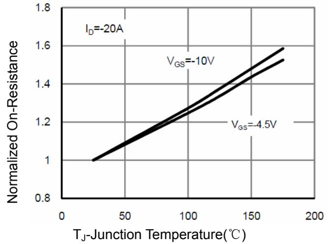
Figure 4 R<sub>dson</sub>-Junction Temperature
