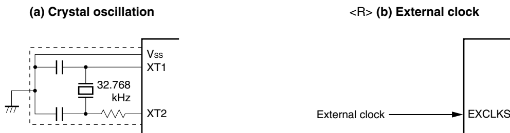
Figure 6-10. Example of External Circuit of XT1 Oscillator
