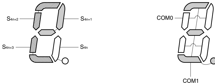
Figure 18-18. Two-Time-Slice LCD Display Pattern and Electrode Connections
