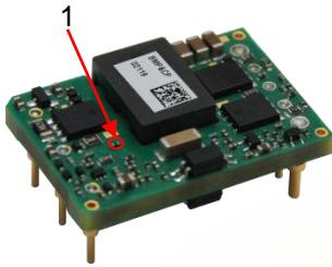
Figure 23: Thermal test point
