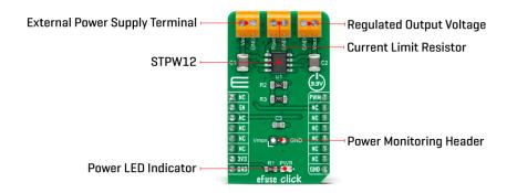
The overcoming of the power limit threshold is signaled on the monitor/fault pin on the onboard header pin labeled as VMON. The monitor/fault pin is proportional to the power, continuously present on the pin, and provides two valuable signals for the real-time control of the device and application status. After a particular delay time, programmable by the user, the STPW12 automatically tries again to close the internal switch and re-connect the load.
