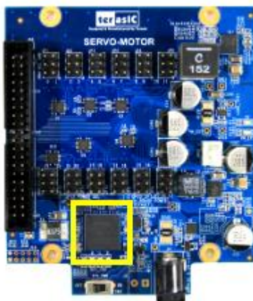
Figure 2-12 CPLD for Power Monitor
