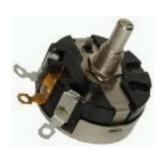
58 Series Industrial Potentiometer, Wire Wound Element, Solder lug Terminals, 4 W Power Rating, 50 Ohm Resistance Value
