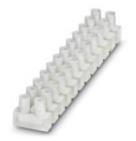
Polyamide Europe terminal strip, transparent, with wire protection, for connecting solid conductors and stranded conductors with and without ferrules with a cross section of 1 to 6 mm<sup>2</sup>
