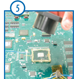
Lift to remove the Knob Tool - leaving the Frame Clip attached to the component.
