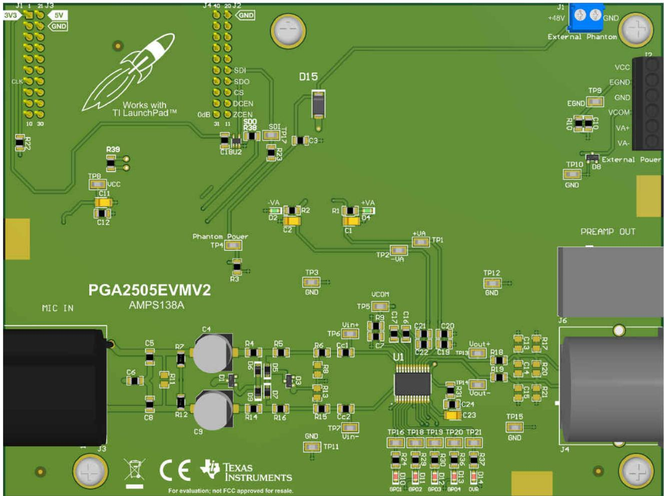
This user's guide describes the characteristics, operation, and use of the PGA2505EVMV2, a refreshed evaluation module (EVM) compatible with the [PGA2505](#) on a modern operating system. This document includes the schematic, printed circuit board (PCB) layout, and bill of materials (BOM). Throughout this document, the terms evaluation board, evaluation module, and EVM are synonymous with the universal PGA2505EVMV2.
