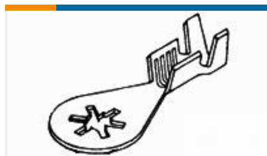
TE Part #640051-1 RING TONGUE .164 18-14 AWG SST
