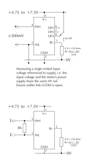
Measuring a current from a circuit which is floating with respect to the DPM's supply, i.e. the current and the meter's power supply are isolated from each other. Ensure solder link LCOM is closed.
