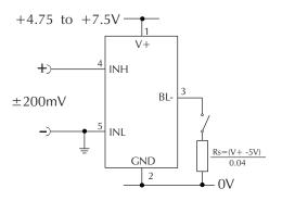
Measuring a single ended input voltage referenced to supply, i.e. the input voltage and the meter's power supply share the same 0V rail. Ensure solder link LCOM is open.
