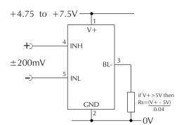
Measuring an input voltage referenced to a floating supply, i.e. the input voltage and the meter's power supply are isolated from each other. Ensure solder link LCOM is closed.
