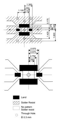
\* Line width to be designed to match 50 ohm characteristic impedance, Depending on PCB material and thickness.
