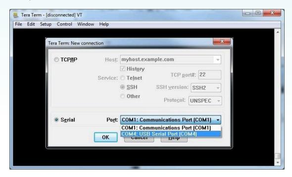
**Note:** Your device may not show up on the port list due to a missing driver. Refer to Section 2.3.1 for instructions on installing a driver.
