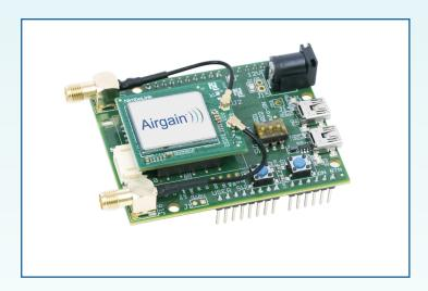
A common issue is accidentally inserting the modem with pins misaligned by one row. Check pin alignment BEFORE applying power to prevent modem damage.
