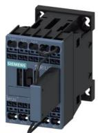
traction contactor, AC-3e/AC-3, 12 A, 5.5 kW / 400 V, 3-pole, 24 V DC, 0.7-1.25\* Us, with integrated varistor, auxiliary contacts: 1 NC, spring-loaded terminal, size: S00, with plugged on series resistor
