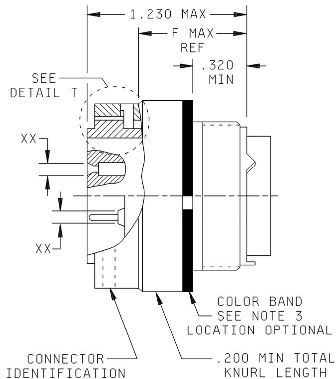
NOTE: For "XX", see note 5 and table I for contact cavities requiring reduced dimensions.
