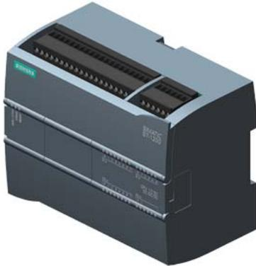
SIPLUS S7-1200 CPU 1215C DC/DC/DC -40...+60°C with conformal coating based on 6ES7215-1AG40-0XB0 . compact CPU, DC/DC/DC, 2 PROFINET ports, onboard I/O: 14 DI 24 V DC; 10 DO 24 V DC; 2 AI 0-10 V DC, 2 AO 0-20 mA DC, Power supply: DC 20.4-28.8V DC, Program/data memory 125 KB
