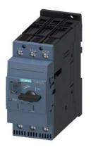
Special type Circuit breaker size S2 for motor protection, CLASS 10 A-release 54...65 A N-release 845 A screw terminal Standard switching capacity Ambient temperature -50 °C 250 switching cycles
