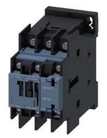
power contactor, AC-3 17 A, 7.5 kW / 400 V 1 NO + 1 NC, 100 V AC, 50 Hz, 100-110 V, 60 Hz, 3-pole, Size S0, ring cable lug connection
