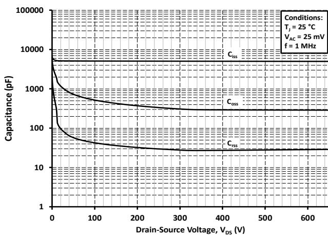
Figure 18. Capacitances vs. Drain-Source Voltage (0 - 650V)
