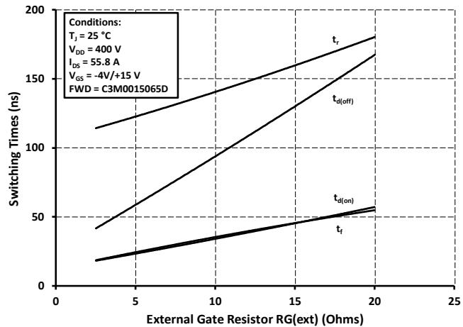
Figure 26. Switching Times vs.  $R_{\text{G(ext)}}$
