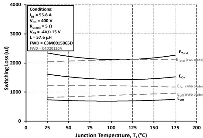
Figure 25. Clamped Inductive Switching Energy vs.
