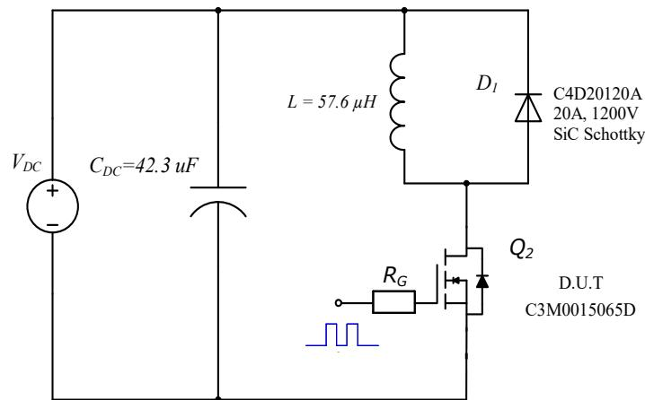
Figure 27. Clamped Inductive Switching
