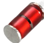
GDT: 2RK075M-4 Size: 4.2*4.0(mm) Working voltage: 75V Nominal withstanding surge current: 3kA(8/20μs)
