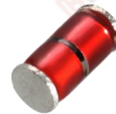
SPG: BK13000702-M Size: 6.0*3.3(mm) Working voltage: 140V Nominal withstanding surge current: 3kA(8/20μs)
