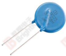
MOV: 101KD14 Size: 14mm Working voltage: 100V
