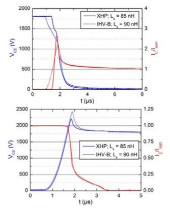
Figure 4: Switching behavior of XHP™ 3 compared to IHV-B, above: turn-on, below: turn-off
