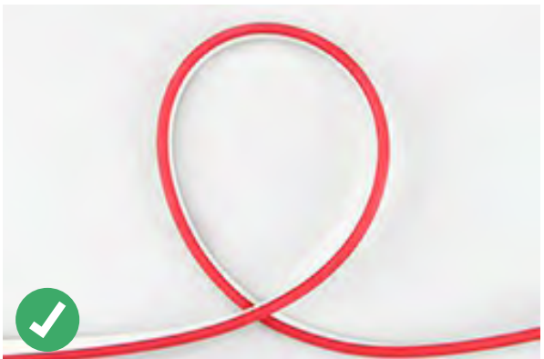
Lighting surface upwards and the strip can be bent to right or left naturally, The minimum bending diameter is 100mm
