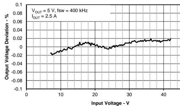
Figure 6. Regulation versus Input Voltage
