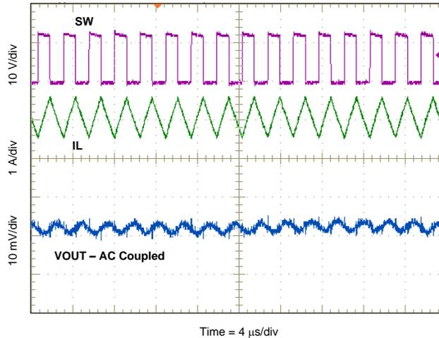
Figure 12. Output Voltage Ripple CCM
