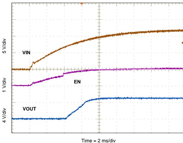
Figure 17. Start Up Relative to  $V_{IN}$  Ramping Up
