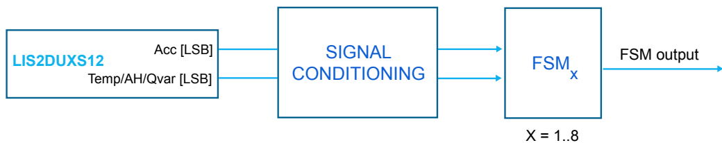
Figure 12. State machine in the LIS2DUXS12
