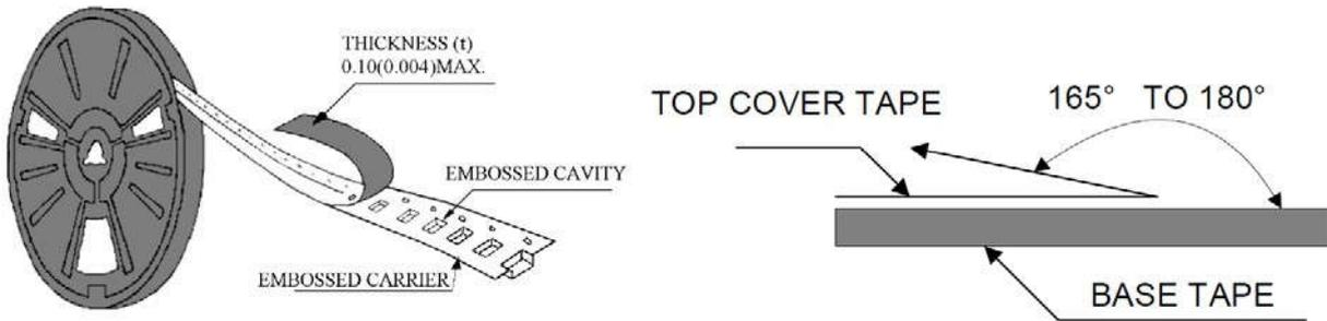
The force for peeling off cover tape is 30 to 100 grams in to arrow direction.
