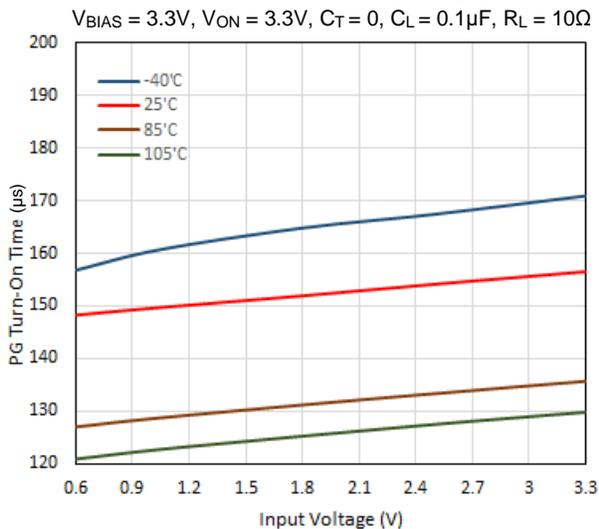
**PG ON Time vs. Input Voltage**
