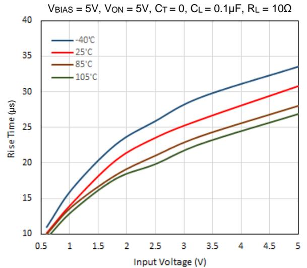
**PG ON Time vs. Input Voltage**
