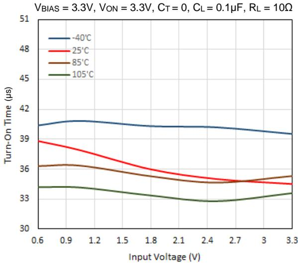
**Turn-ON Time vs. Input Voltage**
