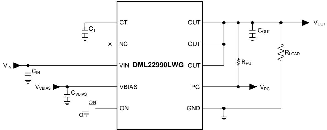
Timing Test Circuit
