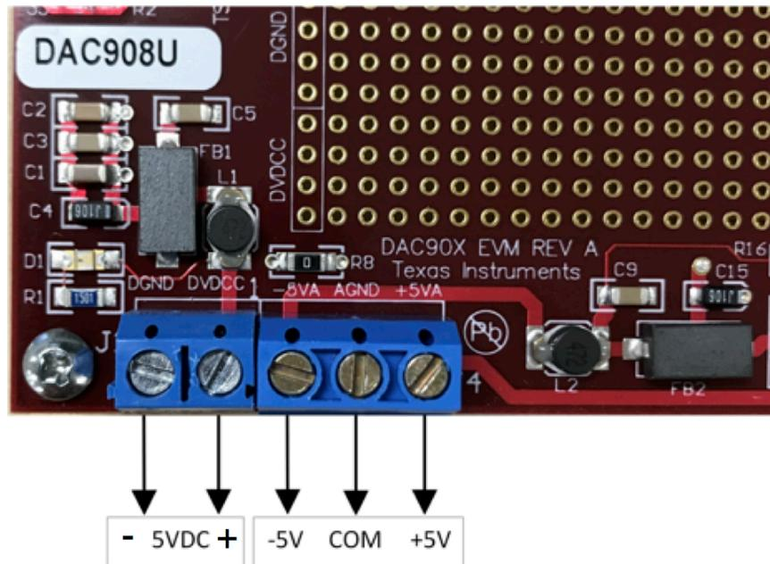
**Figure 4. Power Supply Connections**
