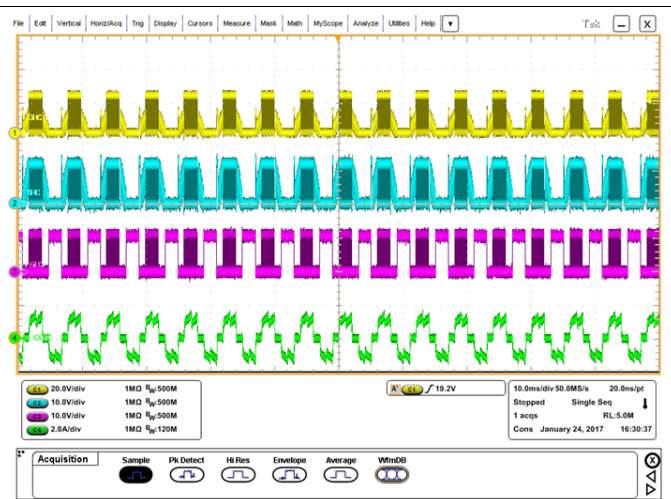
Figure 55. BLDC Motor Commutation 2000 RPM
