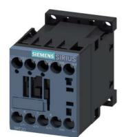
power contactor, AC-3e/AC-3, 9 A, 4 kW / 400 V, 3-pole, 24 V DC, auxiliary contacts: 1 NC, screw terminal, size: S00, communication-capable
