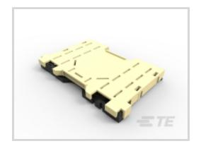
IC Socket Type: LGA 3647 Number of Positions: 1824 Contact Mating Area Plating Material Thickness: [30 µin] Centerline (Pitch): .86 mm, .99 mm [.034 in, .039 in ] Termination Method to PCB: Surface Mount - Solder Ball
