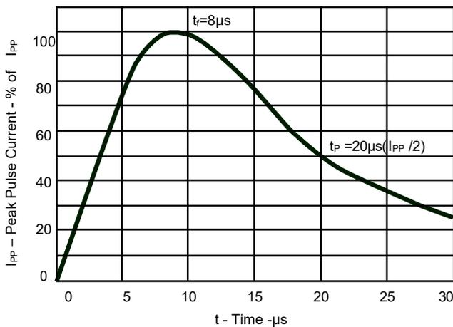
Fig 1.Pulse Waveform
