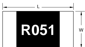
Fig. 5 Chip resistor outlines
