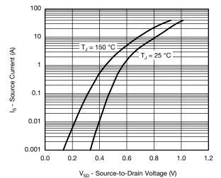
Source-Drain Diode Forward Voltage
