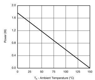
Power Derating, Junction-to-Foot Power Derating, Junction-to-Ambient
