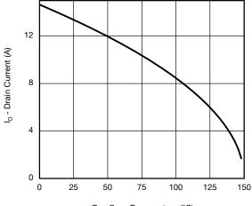
T<sub>C</sub> - Case Temperature (°C) **Current Derating\***
