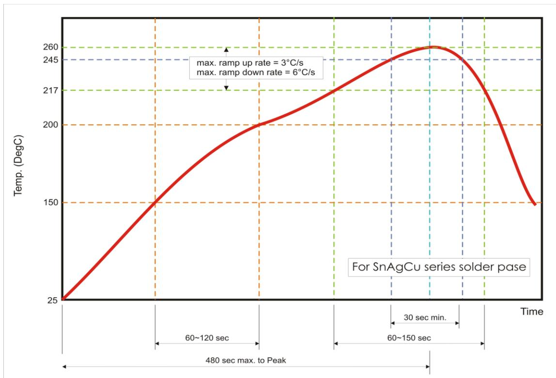
**Fig 3. Infrared soldering profile for Chip Resistors**
