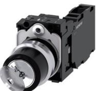
RONIS key-operated switch, 22 mm, round, metal, shiny, lock number SB30, with 2 keys, 2 switch positions O-I, latching, actuating angle 90°, 10:30h/13:30h, key removal O+I, with holder, 1 NO+1 NC, screw terminal, possible special locks: SB31, 421, 455, Z=20-unit packaging
