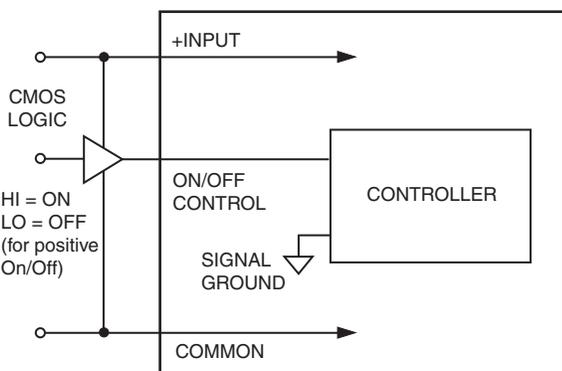
Figure 3. On/Off Control With An External CMOS Gate
