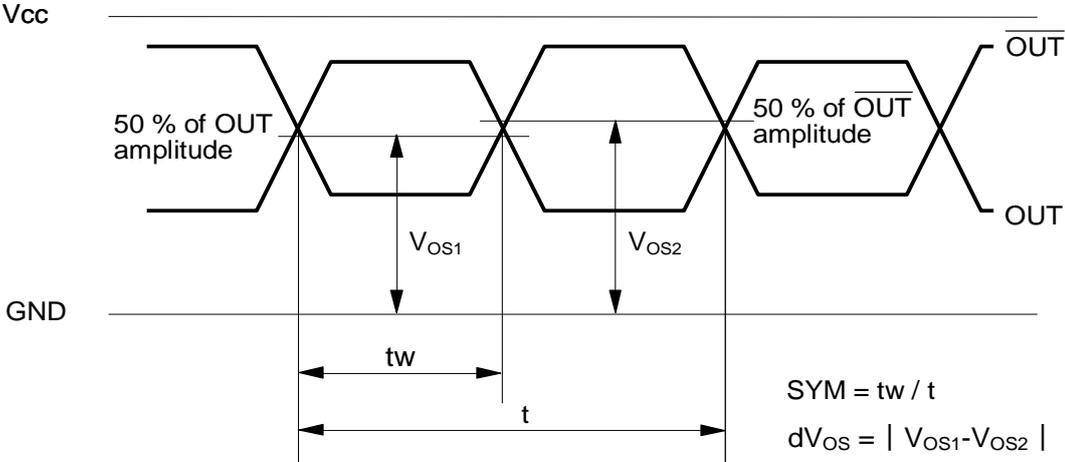
Differential output waveform ( $\text{OUT} - \overline{\text{OUT}}$ )
