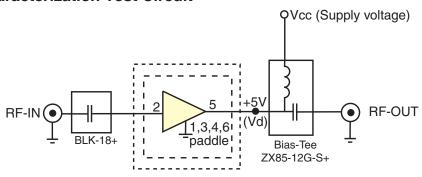
Fig 1. Block Diagram of Test Circuit used for characterization. (DUT soldered on Mini-Circuits Characterization test board TB-640+) Gain, Return loss, Output power at 1dB compression (P1 dB), output IP3 (OIP3) and noise figure measured using Agilent's N5242A PNA-X microwave network analyzer.
