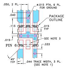
1. TRACE WIDTH IS SHOWN FOR ROGERS RO4350B WITH DIELECTRIC THICKNESS .020" ± .0015"; COPPER: 1/2 OZ. ON EACH SIDE. FOR OTHER MATERIALS TRACE WIDTH MAY NEED TO BE MODIFIED. 2. BOTTOM SIDE OF THE PCB IS CONTINUOUS GROUND PLANE.
