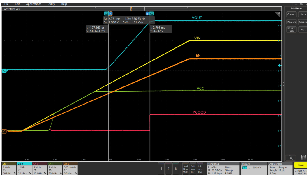
Figure 18 Startup with 4A load (Ch1:PV IN , Ch2: V OUT , Ch3: PGood, Ch4:V CC , Ch5: Enable)
