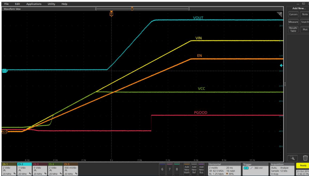
Figure 17 Startup with no load (Ch1:PV IN , Ch2: V OUT , Ch3: PGood, Ch4:V CC , Ch5: Enable)
