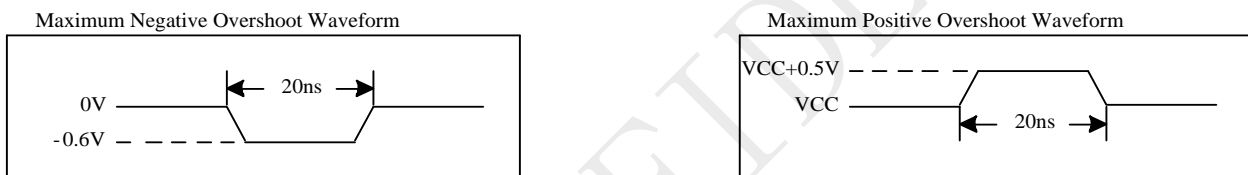
Figure 5-1 Maximum Overshoot Waveform
