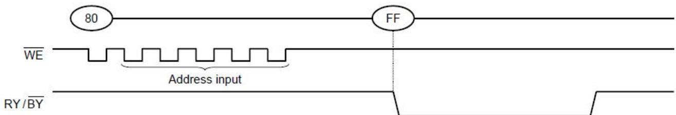
If a command other than “85h”, “10h”, “11h”, “15h” or “FFh” is input, the Program operation is not performed and the device operation is set to the mode which the input command specifies.
