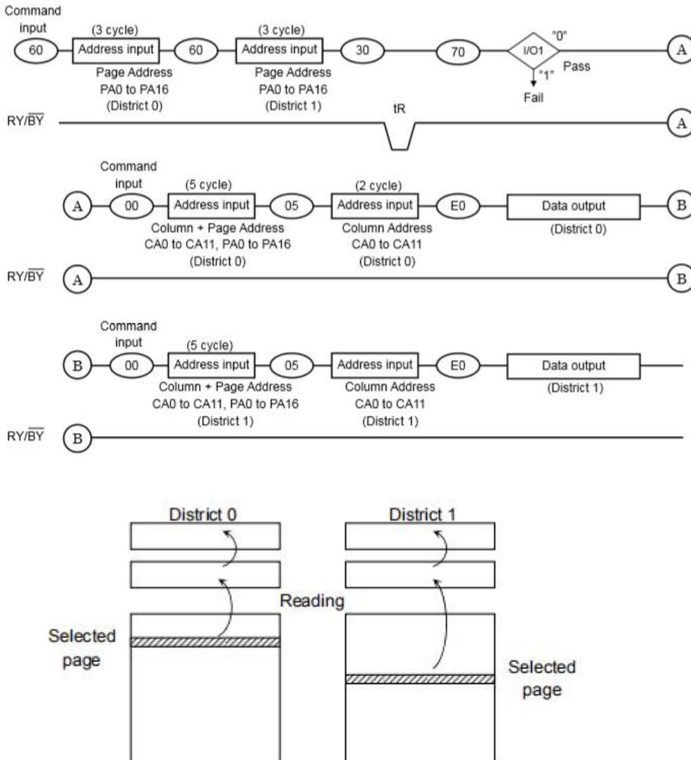
The data transfer operation from the cell array to the Data Cache via Page Buffer starts on the rising edge of  $\overline{WE}$  in the 30h command input cycle (after the 2 Districts address information has been latched). The device will be in the Busy state during this transfer period.
