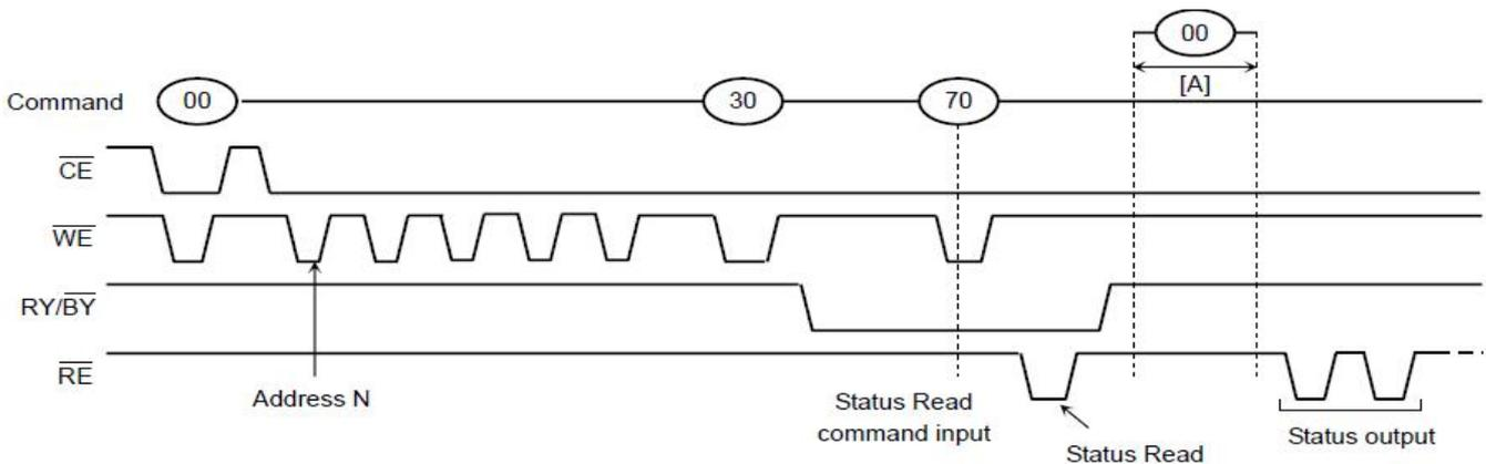
The device status can be read out by inputting the Status Read command “70h” in Read mode. Once the device has been set to Status Read mode by a “70h” command, the device will not return to Read mode unless the Read command “00h” is inputted during [A]. If the Read command “00h” is inputted during [A], Status Read mode is reset, and the device returns to Read mode. In this case, data output starts automatically from address N and address input is unnecessary
