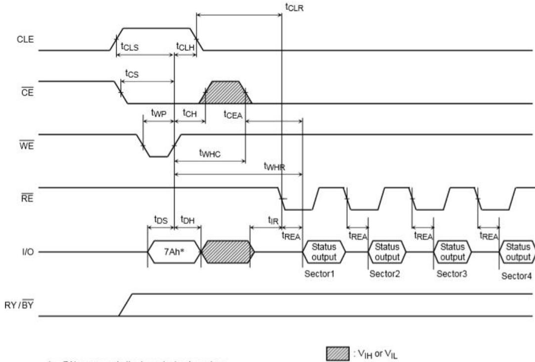
Read Cycle Timing Diagram
