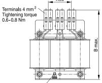
PE M4 / Tightening torque 1.2±0.1 Nm
