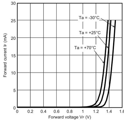
**Fig 3. LED Current vs. Supply Voltage (Typical)**
